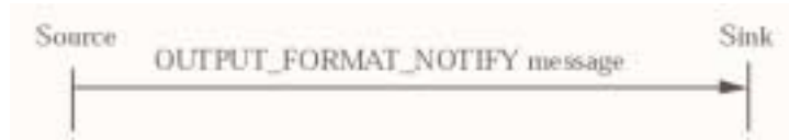
Figure 36: Message sequence for output format data transmission procedure
