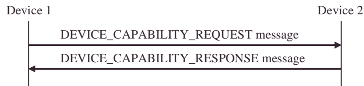
Figure 30: Message sequence for device capability request procedure
