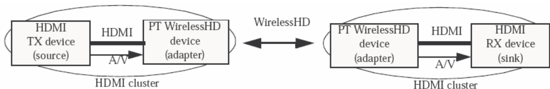
Figure 40: Example of communication between HDMI devices via WirelessHD
